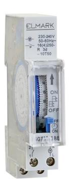
The mechanic relay for time is supposed to be used for managing chains with maximum capacity of 3500W. After the setting, the timer executes the functions we required in 24 hours regime. The minimum period for setting is 15 minutes as it is executed within 96 pcs segments which the timing of the work and rest of the consummator is being set. The timer is accomplished with a battery which assures the work by 70 hours after power failure.
